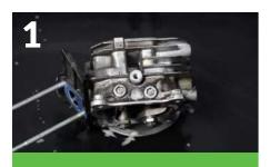
Oil and grease are washed off the dirty part and flow through the Microbial Filter Mat in the sink into the ROwasher tank.
