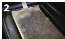
The Filter Mat is the KEY to the system – it contains 200 million oileating microbes and traps particles down to 50 micron.
